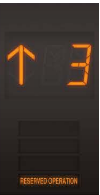
Indicator on car operating panel in the "reserved operation" mode (EXCLC) (Standard)
