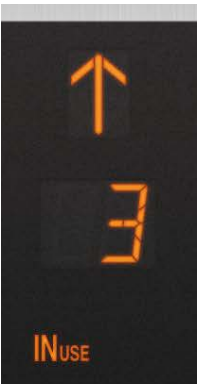
Hall position indicator in the "reserved operation" mode (EXCL) (Standard)
