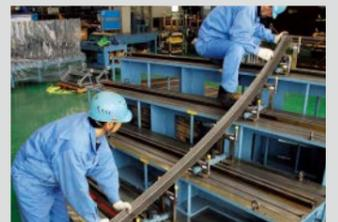
Bending tracks three-dimensionally
